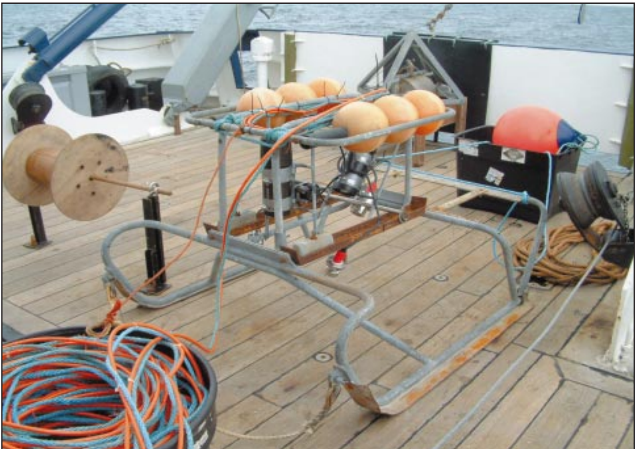
▲ Photosledge with still camera system (black housing) and video camera and lights (red plug retainers), used on the RV Prince Madog cruise. © Crown copyright.
