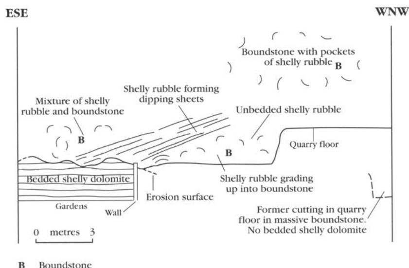
Figure 3.29: Sketch of the stratal relationships in the southern part of the main face of Humbleton Hill Quarry, based on an unpublished drawing made by the writer in 1953.
