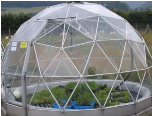
Ozone exposure experiments in solardomes at CEH Bangor. The site was visited during the Network meeting in June 2006. Photograph by Zoe Masters, Natural England. 2006.
