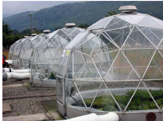
Ozone exposure experiments in solar domes at CEH Bangor. The site was visited during the Network meeting in June 2006. Photograph by Zoe Masters, Natural England. 2006.
