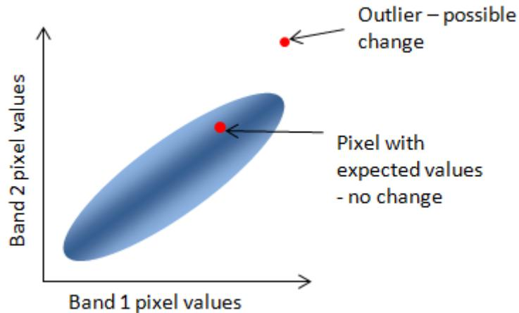
Figure 1: Illustration of the class-specific spectral values for class 1 (blue area) based on two spectral bands and a single outlier (change pixel).
