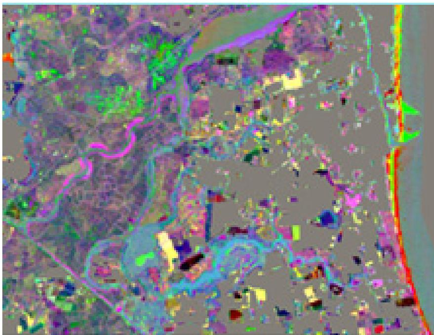
Figure 3: Principal Components Analysis image (bands 4,5,6 as RGB respectively) derived from a 12-band multi-temporal image comprised of the April 2002 and 2011 images.
