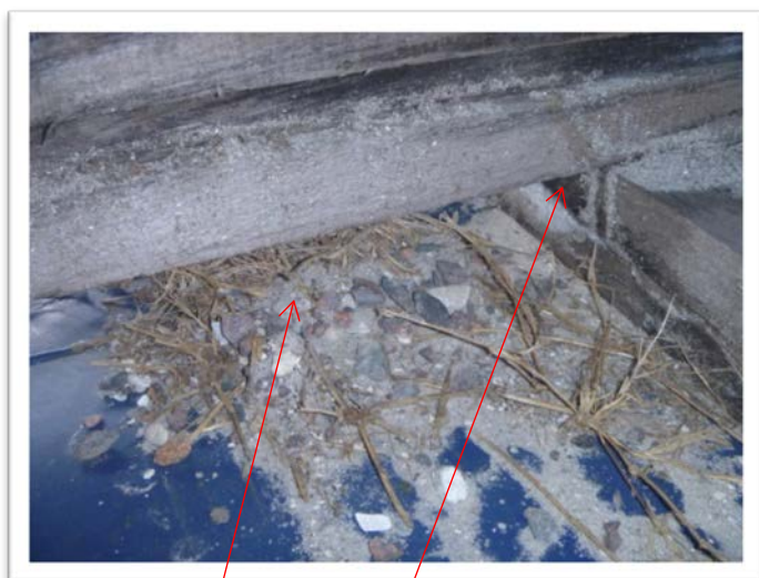
Figure 4. Sand, grass and ant nests as evidence of inadequate cargo storage and inspection prior to loading cargo on to the flatrack
